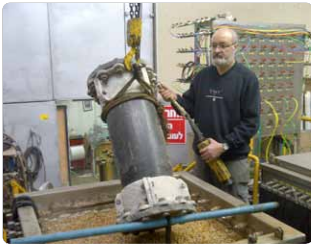
Pressure testing: All pipes undergo strict quality pressure testing
